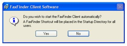
E. The FF240-IP Client software can place a shortcut in the Startup directory so that the client software will start automatically when the PC is booted.
